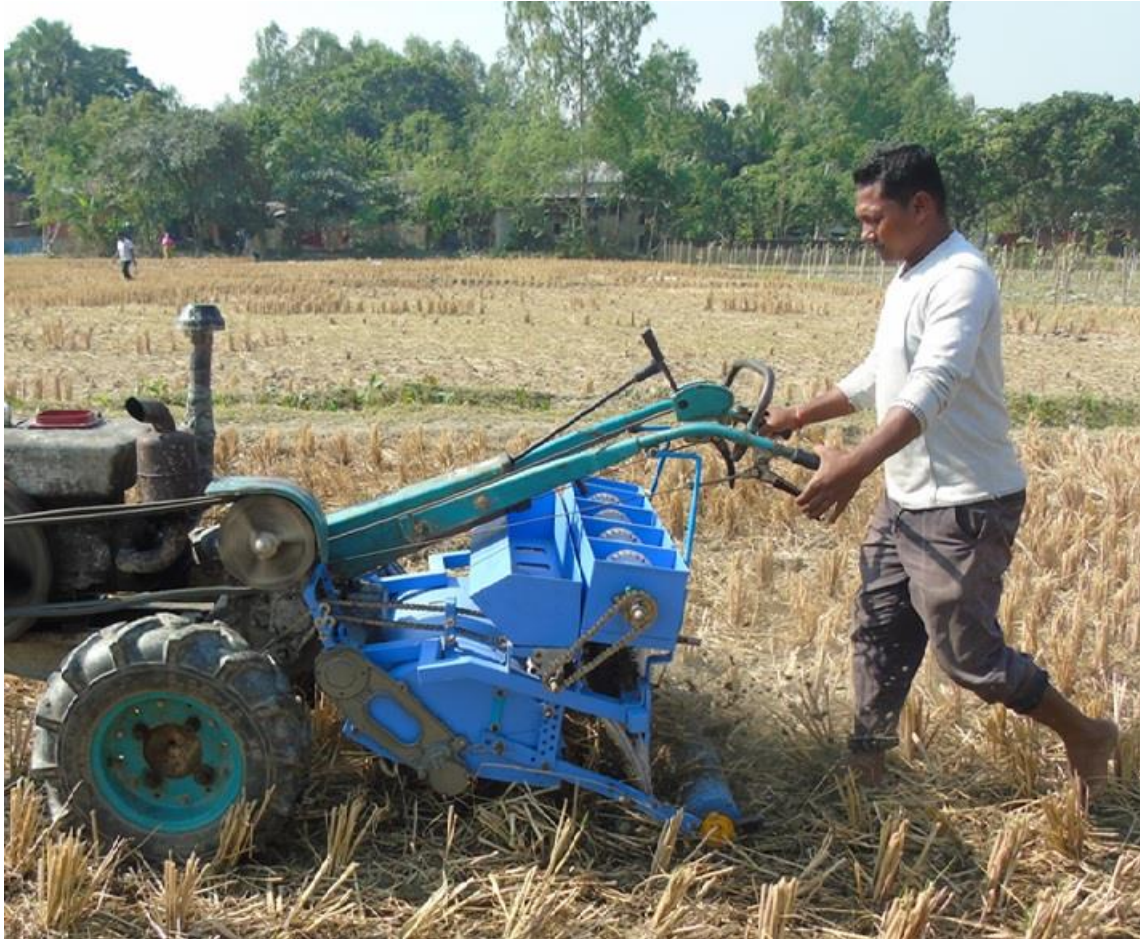
Figure 6.3. A VMP sowing a rabi crop into rice stubble in the HBT. Photo credit: M. Enamul Haque
